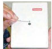
Please note that the pin hole is located on one side of the detector on the 173Mhz version.
