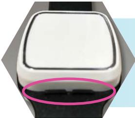
Make sure the black teeth are lined up and fully enclosed to ensure it works properly.
