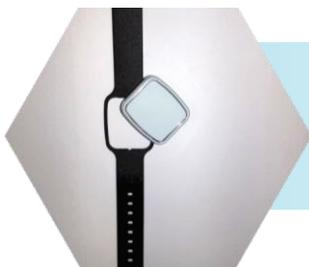
After the retention features, have been removed from both sides of the Vibby; it will easily come out of the wrist strap.
