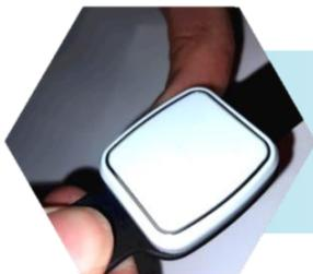
Pull the bottom of the wrist strap onto the Vibby; ensuring the retention features line up with the holes and the edges fall into the enclosure.
