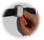
Pull the bottom of the wrist strap onto the Vibby; ensuring the retention features line up with the holes and the edges fall into the enclosure.
