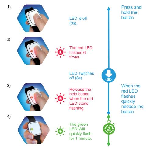
Once the Vibby is in Program Mode it will exit Program Mode automatically after 1 minute. Next move to the 'Configuration Selection' step.
