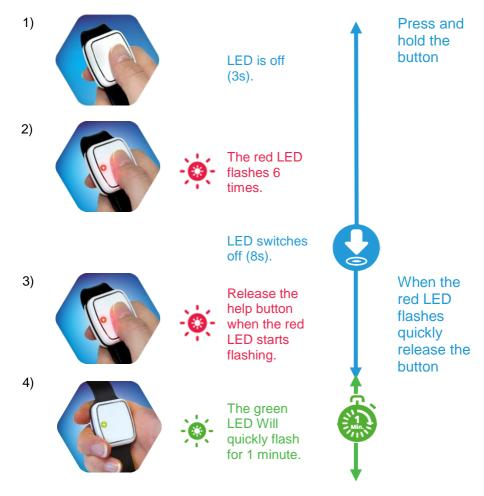
Once the Vibby is in Program Mode it will exit Program Mode automatically after 1 minute. Next move to the 'Configuration Selection' step.
