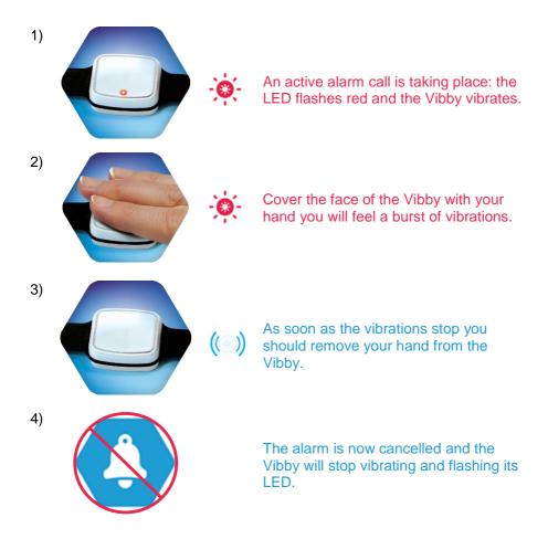
If during step 3, the user does not remove their hand after the first burst of vibrations, the Vibby will vibrate three times to indicate that the alarm has not been cancelled. This is an in-built safety feature that is designed to ensure the alarm is not cancelled if a user covers the Vibby during the fall.
