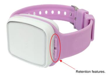
The above diagram shows that the retention features are not installed correctly. Incorrect installation of the Vibby into the wrist strap may cause the Vibby to detach from the wrist/neck cord.
