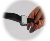
Gently pull the straps backwards to simulate the device being worn on the wrist; this will test if the retention features are correctly inserted within their holes.
