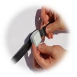
Pull the top of the wrist strap onto the Vibby. Ensuring the retention features line up with their holes and the edges fall within the enclosure.
