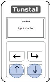
With the LCD activated press and hold the “Up Button” and “Down Button” for 30 seconds.
