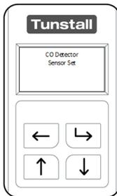
The Universal Sensor will confirm it is now configured to be used with a 3<sup>rd</sup> party device as a CO Detector.
