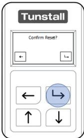
After holding for 30 seconds the LCD will display “Confirm Reset”. Press the “Back Button” to cancel and the “Select Button” to confirm.
