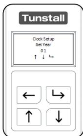
Using the “Up Button” and “Down Button” set the current year and press the “Select Button” to confirm and the back button to exit.
