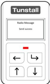
Once the radio message has been sent by the Universal Sensor; it will confirm the status on screen. If **configured** correctly to the Tunstall System this will now receive the transmitted radio message.
