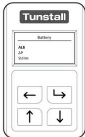
The Battery Menu” has 3 options; **ALB** (auto low battery), **AP** (auto presence) and **Status**. The Universal Sensor must operate in either ALB or AP Mode.
