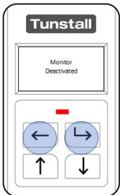
To activate monitoring press and hold the "Select Button" and the "Back Button" together for 3 seconds. The Universal Sensor will confirm that monitoring is activated and will raise an alarm via the Tunstall Home Unit
