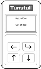
To activate the On/Off Switch, whilst the Universal Sensor is operating in a supported mode press and hold the “Select Button” and the “Back Button” together for 3 seconds.
