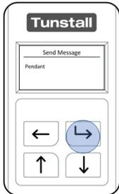
The Universal Sensor will display the available radio message it can transmit, this will depend on the Mode the Universal Sensor is operating in. Press the “Select Button” to send the selected radio message or “Back Button” to exit.
