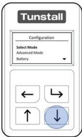
Press the “Down Button” to navigate to the “Send Message” Menu and press the “Select Button”.
