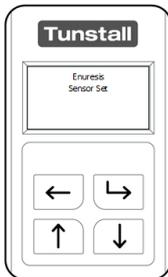
The Universal Sensor will confirm it is now configured to be used with a 3<sup>rd</sup> party device as an Enuresis Sensor.
