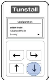
Press the “Down Button” to navigate to the “About” Menu and press the “Select Button”.
