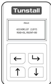
After displaying the installed firmware version; the Universal Sensor will timeout of the “About Menu” after 5 seconds will return to the “Configuration” Menu.
