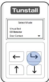
When **“CO Detector”** is highlighted press the **“Select Button”**
