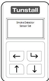
The Universal Sensor will confirm it is now configured to be used with a 3<sup>rd</sup> party device as a Smoke Detector Sensor.
