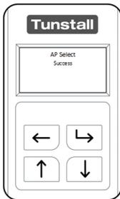
On supporting Tunstall systems, Auto Presence provides additional checks to provide reassurance that the Universal Sensor is functioning. When AP is active the Universal Sensor sends a signal to the home unit every 4 hours.
