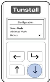
Press the “Down Button” once to navigate to the “Advanced Mode” Menu and press the “Select Button”.
