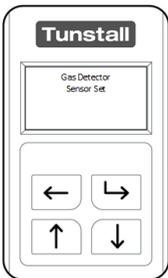
The Universal Sensor will confirm it is now configured to be used with a 3<sup>rd</sup> party device as a Gas Detector.
