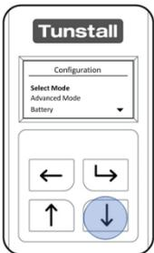
The “Select Mode” menu will be highlighted when first opening the “Configuration Menu”, press the “Select Button” to enter “Select Mode”.
