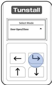
When "Door Contact" is highlighted press the "Select Button"
