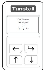
Using the “Up Button” and “Down Button” set the current month. (months 01-12) and press the “Select Button” to confirm.
