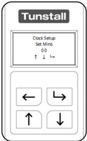
Using the “Up Button” and “Down Button” set the minutes of the current time. (00-59) and press the “Select Button” to confirm.
