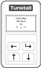
Using the “Up Button” and “Down Button” set the time starting with hours. This is a 24-hour clock. (00-23) and press the “Select Button” to confirm.
