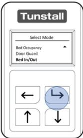
After **unlocking** the Universal Sensor and entering **“Select Mode”** navigate the menu using the “Up Button” and or “Down Button”
