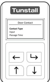
The “Advanced Menu” options depend on which Mode has been configured within the “Select Mode” Menu of the Universal Sensor. For more details on each Mode’s advanced menu, see section 4. Operating Modes.
