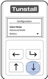
Press the “Down Button” twice to navigate to the “Battery” Menu and press the “Select Button”.
