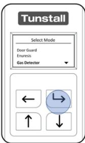
When **“Gas Detector”** is highlighted press the **“Select Button”**
