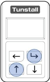
Then press and hold the "Up Button" and the "Select Button" until 'Change Settings' appears on the display.
