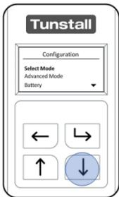
Press the “Down Button” to navigate to the “Setup Summary” Menu and press the “Select Button”.
