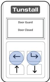
In **Door Guard** Mode it is possible to stop the Universal Sensor from sending alarms to the Tunstall Home Unit by deactivating it for a pre-determined period.
