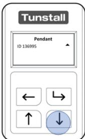
Pressing the “Down Button” will then display the Sensor ID. After 8 seconds the Universal Sensor will revert to the “Configuration Menu”.
