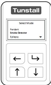
When “Smoke Detector” is highlighted press the “Select Button”
