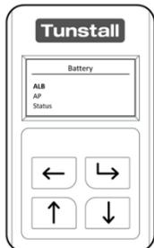
The Battery Menu” has 3 options; **ALB** (auto low battery), **AP** (auto presence) and **Status**. The Universal Sensor must operate in either ALB or AP Mode.
