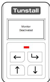
TO deactivate press and the hold the "Select Button" and the "Back Button" together for 3 seconds. The Universal Sensor will confirm that monitoring has been deactivated. The red LED will flash every 30 seconds. After the chose time out the Universal Sensor will begin monitoring again.
