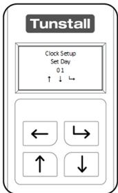
Using the “Up Button” and “Down Button” set the current date. (day 00-31) and press the “Select Button” to confirm.
