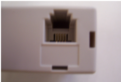
This is a view of an RJ11 Socket
