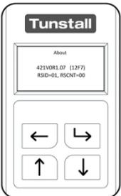
After displaying the installed firmware version; the Epilepsy Sensor Transmitter will timeout of the "About" Menu after 5 seconds and will return to the "Configuration" Menu.
