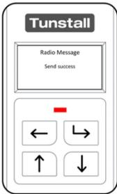
Once the radio message has been sent by the Epilepsy Sensor Transmitter; it will confirm the status on screen. If **configured** correctly to the Tunstall System this will now receive the transmitted radio message.
