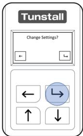
Press the "Select Button" to confirm you want to unlock the sensor.
