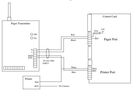
IMPORTANT - if a system printer is also fitted then the printer RTS signal (normally connected to PBY) MUST be disconnected.
