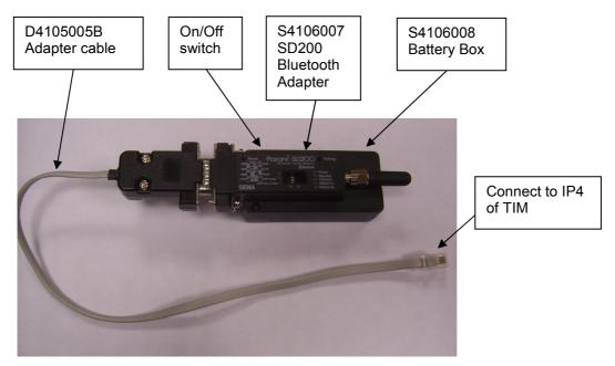
The above picture shows the Parani SD200, battery box and cable assembly that is used to allow the TIM to connect to the Palm personal organiser using Bluetooth.
