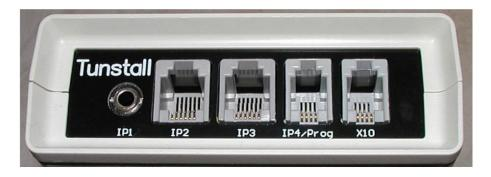
IP1 is used to connect the keyswitch (41005/08) using the cable (D4105004B)
