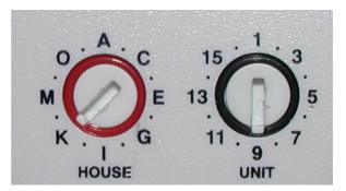
To set the address, simply insert a broad bladed screwdriver into the slot on the rotary switch, until the switch points to the desired address.
