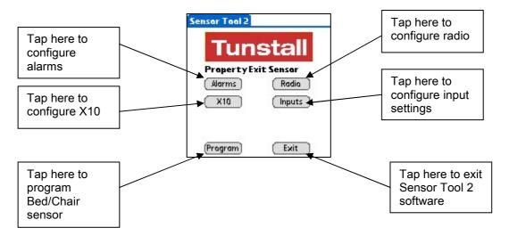
Tapping the Alarms, X10, Radio and Inputs buttons will move to the relevant configuration screen for that part of the PES functionality. Each of these screens has a Back button that will move back to the main options screen. Tapping the 'Program' button will write the new settings to the PES. Tapping the Exit button will exit the Sensor Tool 2 software.
