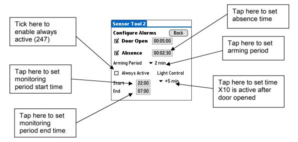
Note that if the Always Active checkbox is ticked then the monitoring period and light control settings are hidden. The Absence time is the time a client can be absent from the property. The Arming Period is the length of time, the PES waits before restarting monitoring after the keyswitch is moved to the enable position e.g. after a carer has left the property. The Light Control value is the length of time, an X10 controlled appliance remains on after the door has been closed.
