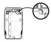
Press and hold down the volume button using a pen/pencil. A beep will be heard when all sensors have been removed.
