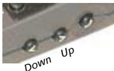
*The volume received at the handset is adjustable using the keys shown. The Resident's Speech Module sound levels can also be adjusted at Communicall by pressing '8' followed by '#' to turn sound up or '9' followed by '#' to turn the sound level down.*
